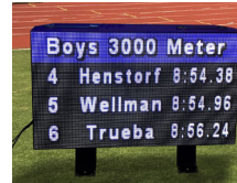
3.2"W x 1.6"H 5mm Portable LED Display
