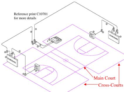
Plug a control into both jacks for Main Court "All-on" operation (shown) or plug two controls into each jack for independent cross-court operation (not shown).
