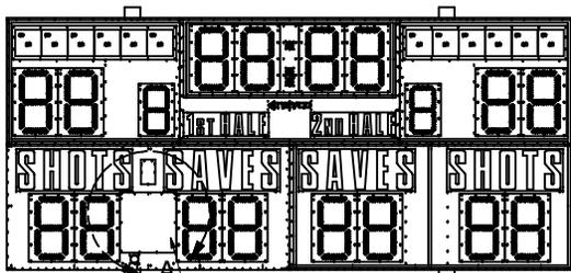
Locate removable door on scoreboard. Remove door and remove cover of electrical enclosure to make connections shown to right.
