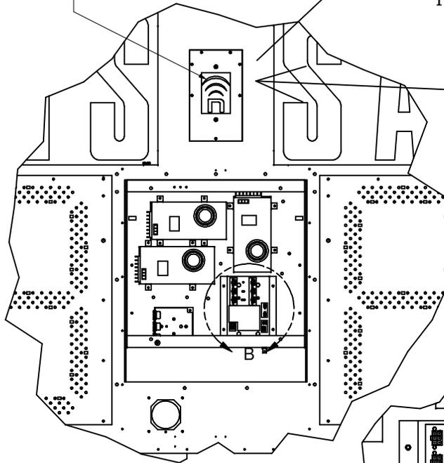
Connect cable to receiver assembly and mount receiver assembly using existing screws
